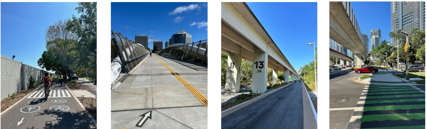
Figure 62 Examples of Trail Wayfinding Design: Pedestrian Crossing (left) Modal separation (center), Mile marking on elevated structure, Green pavement crossing treatment. (Source: Arlington County)
