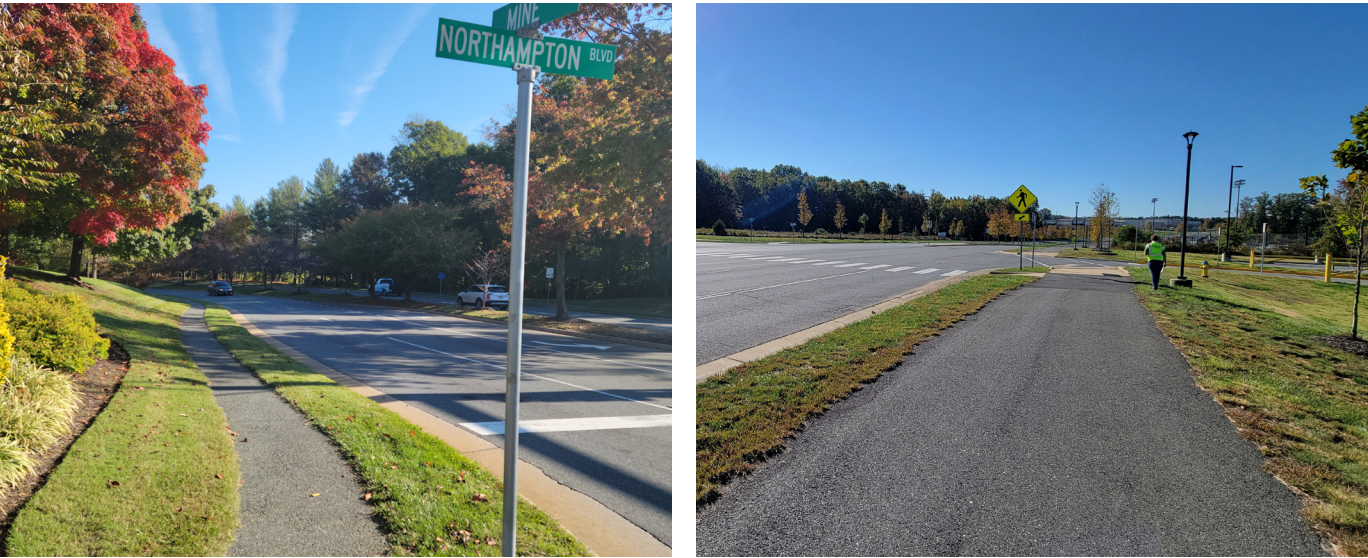
Figure 46: Narrow shared use path along Mine Road at Northampton Boulevard (left) and wide shared use path along Mine Road at Shields Road (right)
