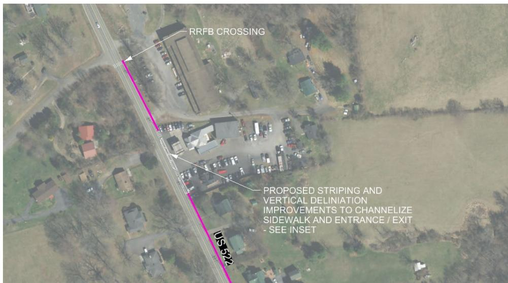
*Figure 3. Proposed Striping and Vertical Delineation at Settle's Grocery and Garage in Flint Hill*
