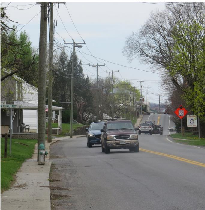
**Figure 2: Sidewalk Obstructions Along US 11 in the Town of Mount Crawford.**
