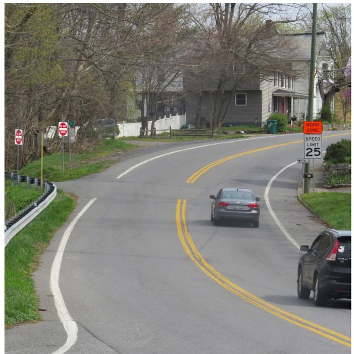
**Figure 3: Unmarked Crossings and Lack of Pedestrian or Bicycle Facilities Along US 11 Between the Town Southern Limit and the Intersection with Mill Street.**
