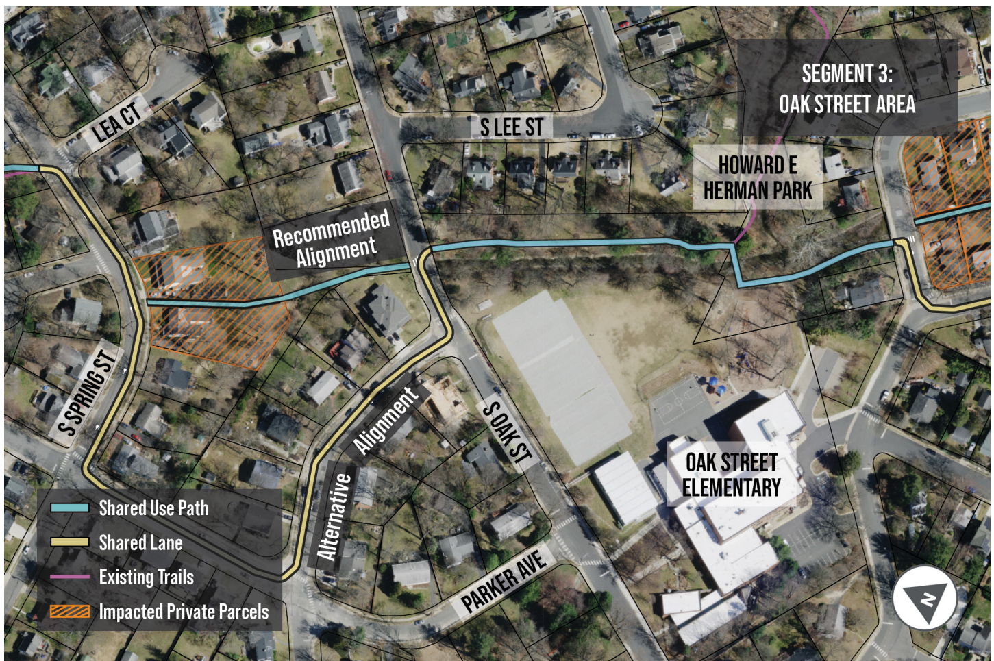
Figure 28. Segment 3 Recommended and Alternative Alignments
