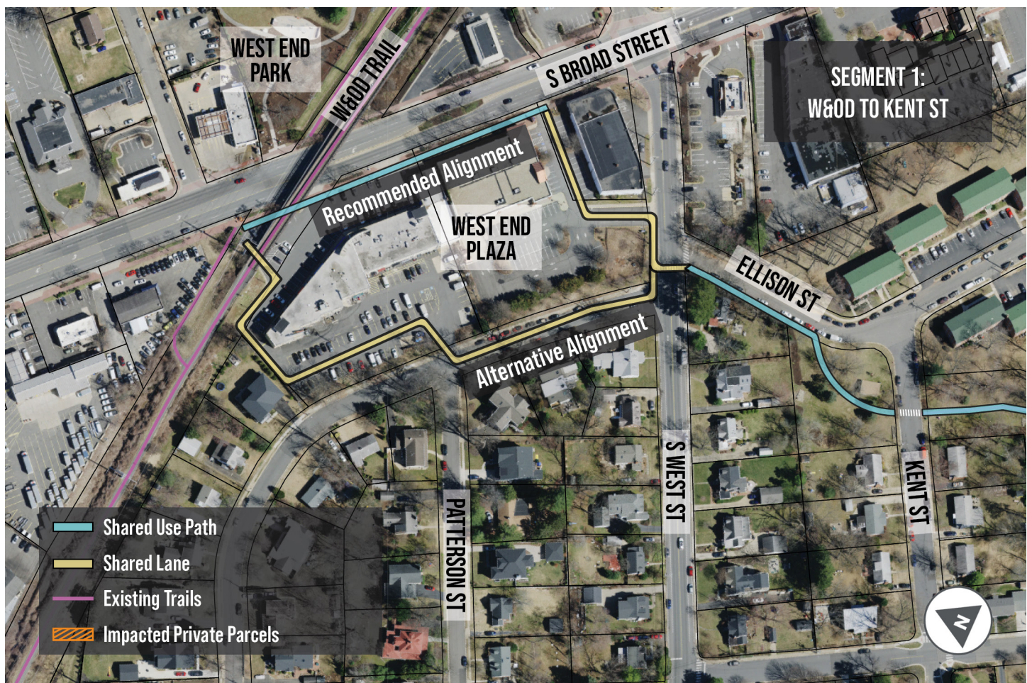
Figure 16. Segment 1 Recommended and Alternative Alignments
