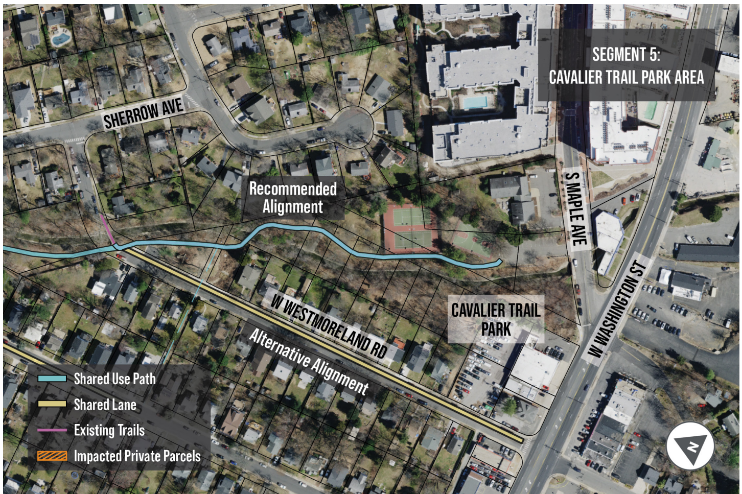
Figure 35. Segment 5 Recommended and Alternative Alignments
