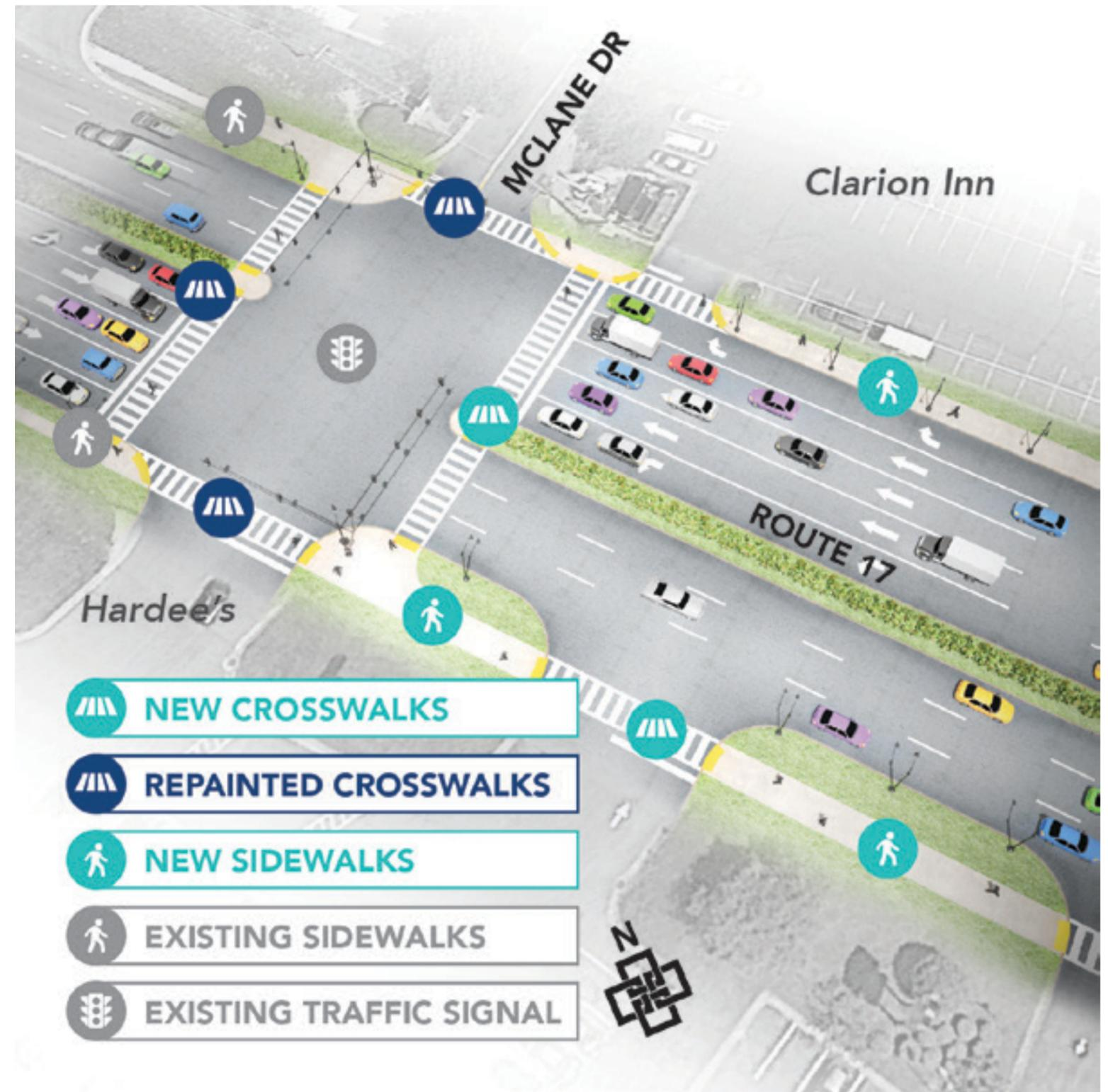
Figure 14: Map of Crosswalk, Sidewalk, and Signalized Intersection Needs Along Gap 1
