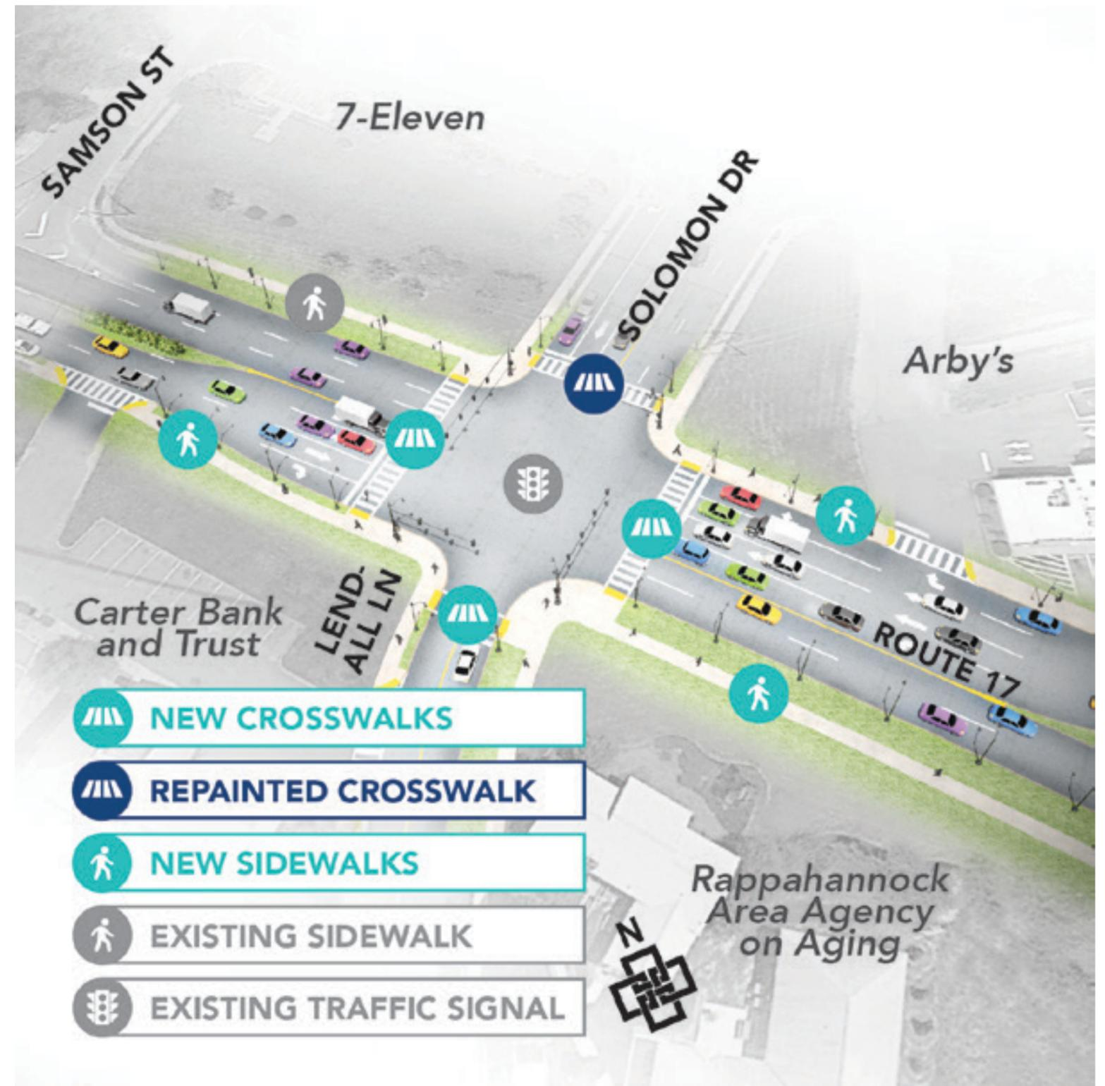
Figure 15: Map of Crosswalk, Sidewalk, and Signalized Intersection Needs Along Gap 3
