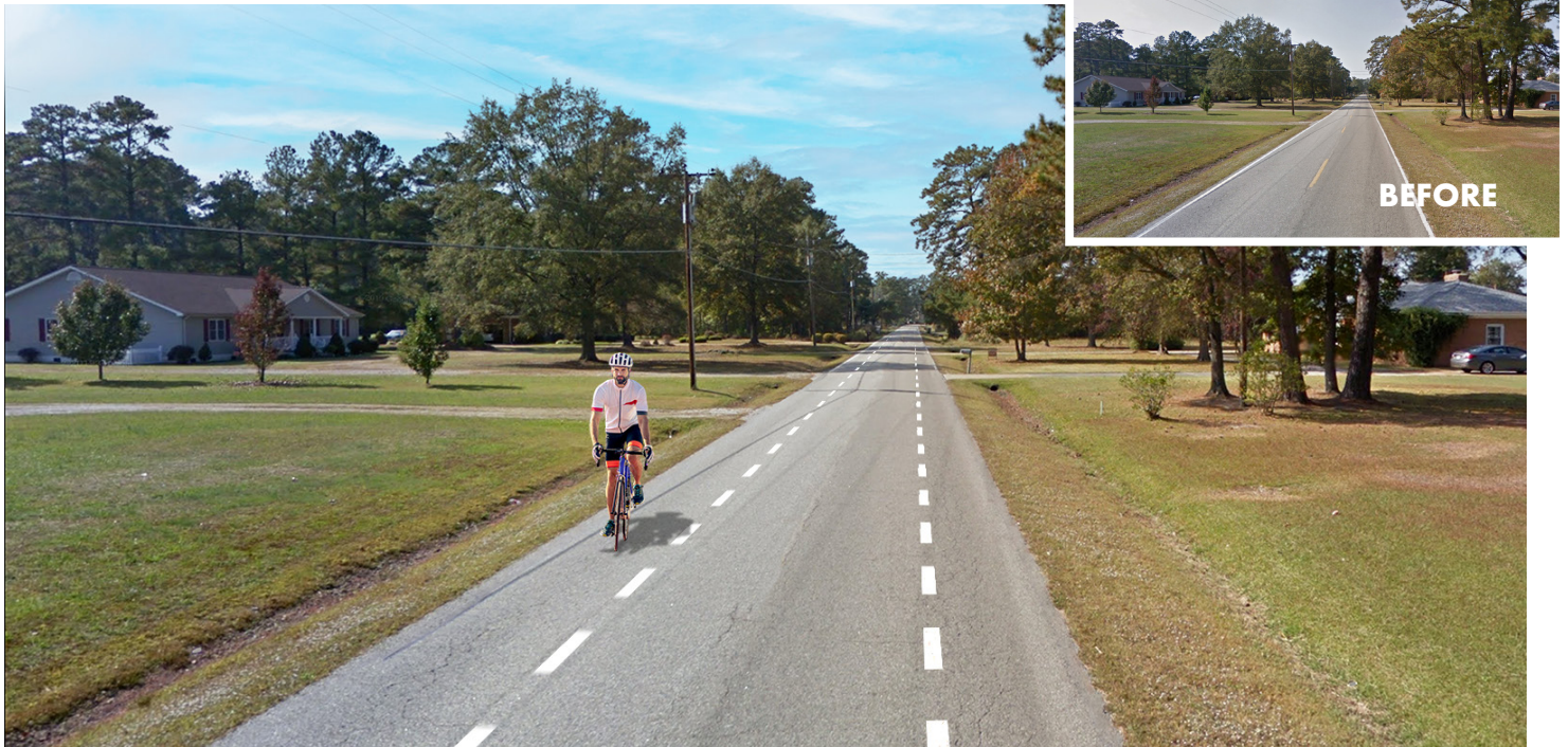
Figure 22: Illustration of the Advisory Shoulder treatment that may be considered along the “Guinea Loop”
